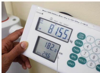
Two LCD screens for easy reading of weight, height, BMI
