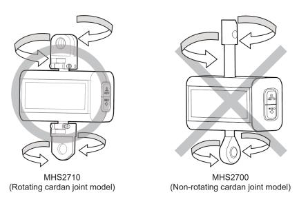
The cardan joints on MHS2710 Lift Scales (with **rotating** cardan joints) will swivel, but only **horizontally**. If they can be manually twisted in any other direction, that means joints are damaged, and the Lift Scale should NOT be used Scale.
