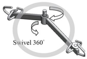
Even if the MHS2710 Lift Scales with horizontally-rotating cardan joints are used, rotation should be conducted by the Patient Lift System, and not the Lift Scale, to minimize risk of damage to Lift Scale.
