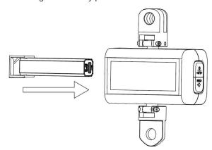
When power is low, please recharge the battery pack using the micro-USB port. When the port light is blinking **red**, battery is being charged. When the port light is stable **green**, battery is fully charged.
