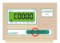
To count items on the scale, first place a sample quantity on the scale. Switch the indicator to count mode by pressing FUNC, holding the button until 'COUNT' is displayed
