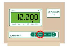
You can use the scale to total up several loads. Add your first item to the scale and press ACCUM. Remove the item from the scale.
