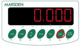
To clear accumulated readings press ZERO.
