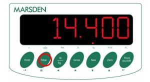
You can use the scale to total up several loads. Add your first item to the scale and press TOTAL. Remove the pallet from the scale.
