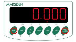
Press PRINT/ON/OFF once and HOLD twice to set the time out period and return to normal weighing mode.
