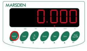
Press HOLD to return to normal weighing mode.
