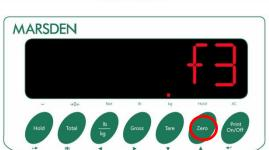
To save battery power, the screen can power off after a set period of time. To set the time out function, with the indicator switched on and nothing on the scale, press and hold HOLD until 'F1' is displayed.
