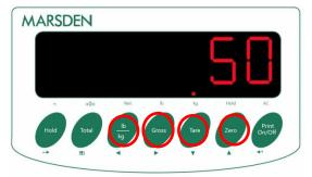
Use the LB/KG and GROSS keys for left and right and TARE and ZERO as up and down to input the sample size.
