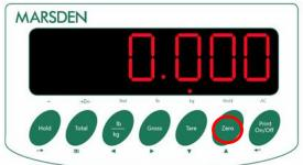
To clear accumulation readings press ZERO.
