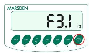
Press PRINT/ON/OFF, and F3.1 should appear on the screen. Press PRINT/ON/OFF again.
