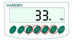
Use LG/KG, GROSS, TARE and ZERO as arrow keys to select the power-off delay (up to 60 mins).
