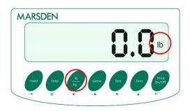
To switch the weight reading between kg and lb, press LB/KG.
