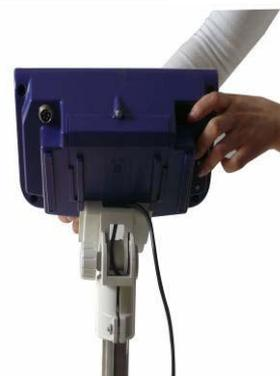
Step 4: After connecting load cell connector to load cell port, the installation is completed.
