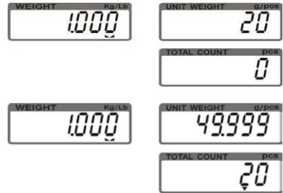
The unit weight is calculated, with Symbol “▼” Pointing at “ACAI”.
