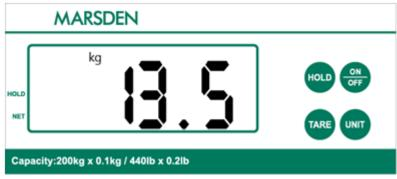
The display will show 0.0 and an arrow should appear pointing to **NET**. This indicates that tare is active. If you remove the item, it should display a negative number.
