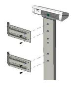
Using the four M5\*0.8\*9 screws provided, mount the two brackets onto the column of the M-110.
