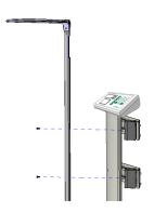
Using the two M6\*1.0\*10 screws provided, screw the HM-201M to the black blocks.
