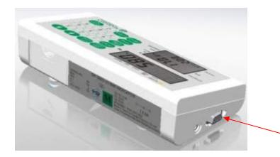
Plug the cable to the printer, and then connect its 9D connector to the indicator.
