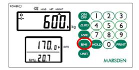
Weigh the patient as normal. The display will show the weight, height and BMI value. At this time, the weight and height can be freely changed, and the BMI value will be automatically calculated according to the changed weight and height.
