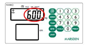
After a few seconds the scale will lock on the person's weight. When the patient leaves the scale, the weight will remain on the display.
