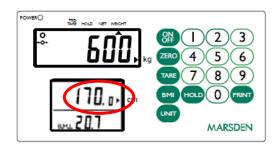
The display will show the last height entered and the extreme left digit will flash. Enter the height by using the numeric keys.\* Press ZERO to confirm the height. (NB: There will always be an active flashing digit in the height display, unless HOLD is pressed).
