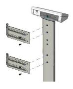
Using the four M5\*0.8\*9 screws provided, mount the two brackets onto the column of the M-110.
