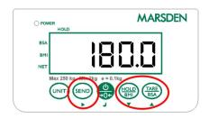
Enter the height by using the TARE/BSA button to decrease the value and HOLD/BMI button to increase the value. To move to the next digit, press SEND.
