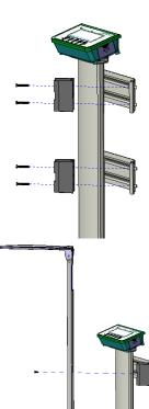
Using the four M5\*0.8\*25 screws provided, screw the black blocks onto the mounting brackets.
