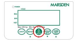
Press the ON/ZERO/OFF button firmly.
