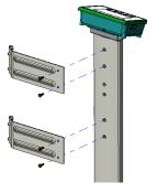
Using the four M5\*0.8\*9 screws provided, mount the two brackets onto the column of the M-125.
