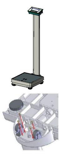
Position the column so that it is resting on the base, ensuring all wiring from the base to the indicator is safely tucked inside the column housing.
