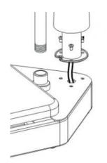
5) Push the height rod through the hole at the base of the indicator and then connect to the black stopper on the base of the scale. Rotate the height measure clockwise to screw into the base.
