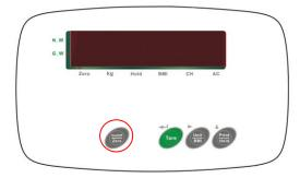
To turn the scale on press the ON button firmly.
