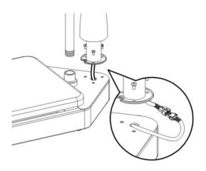
4) Fix the column onto the scale base using the 3 x M5 bolts, making sure not to trap any wires.
