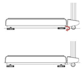
3) Ensure that all four of the levelling feet and the wheels are firmly on the ground and that the spirit level bubble is located in the center as shown below:
