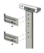
Using the four M5\*0.8\*9 screws provided, mount the two brackets onto the column of the M-160.
