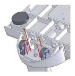
Holding both the column and the base, ensuring all wiring is tucked inside the column housing, turn the scale over so that the column can be screwed to the base from the underside of the base.
