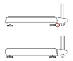
3) Ensure that all four of the levelling feet and the wheels are firmly on the ground and that the spirit level bubble is located in the center as shown below:
