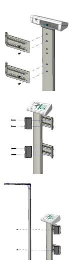
Using the four M5\*0.8\*9 screws provided, mount the two brackets onto the column of the M-165.
