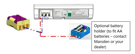
4. Place the housing back in the back of the indicator, and close the battery housing cover.
