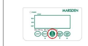
Hold the ON/ZERO/OFF button for three seconds when the scale is turned on. The scale will power down.
