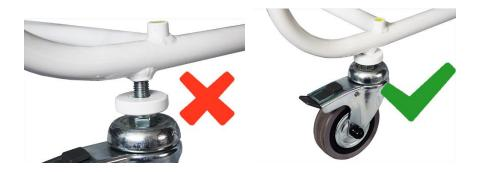
For safety, at least 15mm of thread should always be inside the frame of the scale
