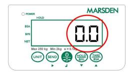
When the scale shows 0.0 on the display you are ready to start weighing.
