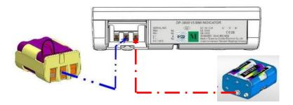
Place the housing back in the back of the indicator and close the battery housing cover.
