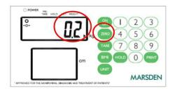
If for any reason the scale shows a reading other than 0.0kg it can be reset to zero.
