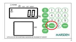
Press HOLD again to disable the Hold function and return the scale to 0.0kg.
