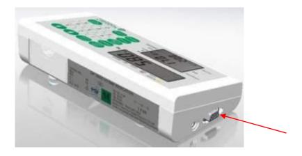
Plug the cable to the printer, and then connect its 9D connector to the indicator.
