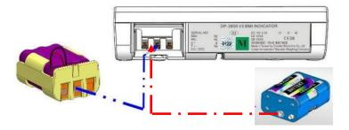
4. Place the housing back in the back of the indicator and close the battery housing cover.
