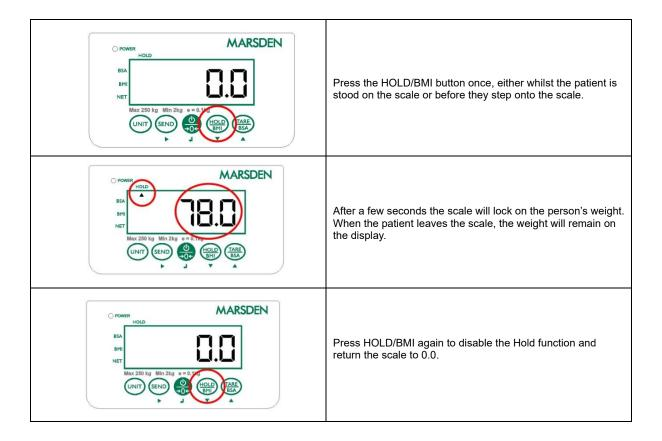
Note: If the weight reading remains on the display for more than five minutes, the Hold
