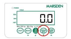
Press the HOLD/BMI button once, either whilst the patient is stood on the scale or before they step onto the scale.
