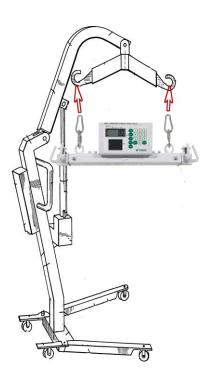
5. Place the patient in the sling and attach the sling loops onto the hooks on both sides of the hoist weighing attachment. The design and procedure may vary depending on the different sling makers. Please refer to the instructions provided by the sling manufacturer.
