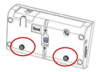
2. Mount the indicator to the front of the hoist attachment. Secure in the position shown using the two thumb screws.
