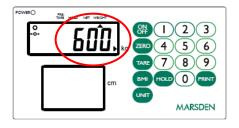
After a few seconds the scale will lock on the person's weight. When the patient leaves the scale, the weight will remain on the display.
