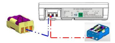
Place the housing back in the back of the indicator and close the battery housing cover.
