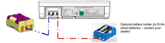
Place the housing back in the back of the indicator, and close the battery housing cover.
