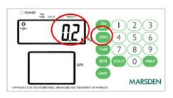
If for any reason the display shows a reading other than 0.0 when there is nothing on the scale it can be reset to zero.
