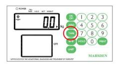
To use the Tare function, add the item you wish to tare off to the scale, and press TARE. The display will show zero, and then a minus number when the item is removed from the scale. Press HOLD for three seconds to access the time setting mode. The time period digit that is flashing can be changed by entering the appropriate number from the numeric key pad. The time period to be edited is selected by pressing HOLD.
