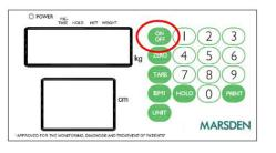
Press the ON/OFF button when the scale is turned on. The scale will now power down.
