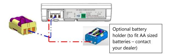
4. Place the housing back in the back of the indicator, and close the battery housing cover.
