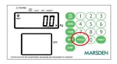
With the scale on and pads next to castors, press the HOLD button.
