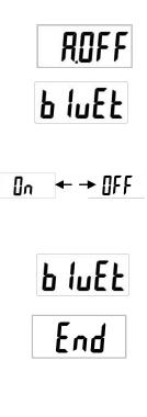
Long press ZERO for three seconds to enter the Setting mode and then display the A-OFF menu.
