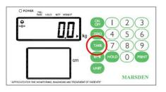
Press TARE for three seconds to enter Preset Tare setting mode.
