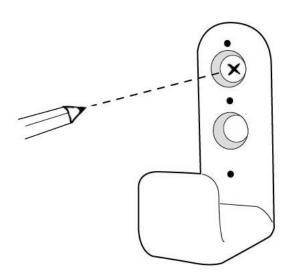
Drill two 6.5mm the holes for each hook.
