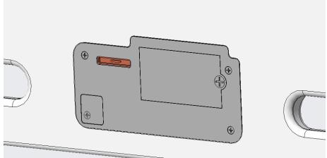
The port for the charging cable is magnetic. Clip the end of the cable in place and plug the other end of the cable into a power socket. Please do not use any form of charging cable other than the one supplied with the scale. The scale cannot be used whilst recharging.
