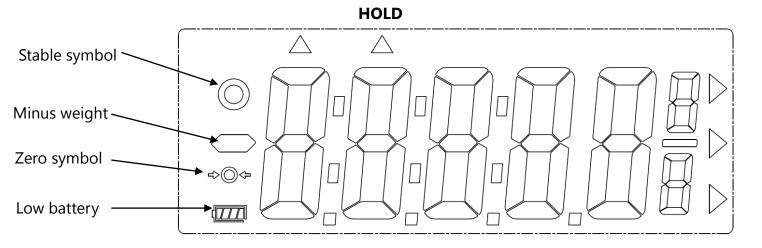
Stable symbol: To indicator the weight reading is stable
