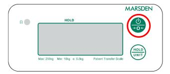
Press and hold ON/OFF/ZERO button for three seconds to power the scale down.
