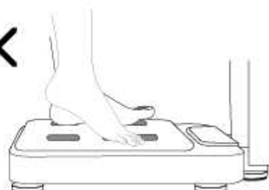
Incorrect foot electrode contact
