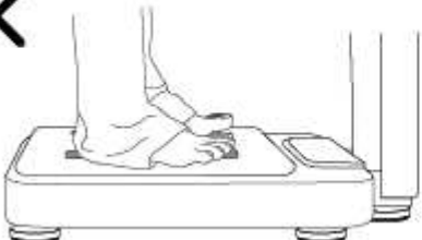
Heels are obstructed from full contact with rear electrodes due to clothing.
