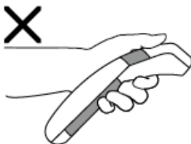
Thumb not in contact with thumb electrode
