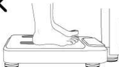
Feet are not in full contact with rear electrodes
