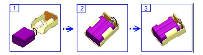
2. Place the battery housing back making sure that the housing pin is connecting to the right point.
