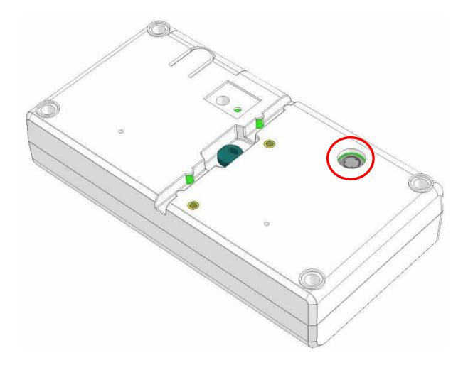
Insert the HM-201D data cable into the socket of the indicator before use.
