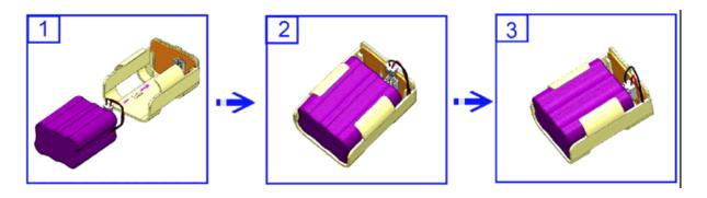
2. Place the battery housing back making sure that the housing pin is connecting to the right point.
