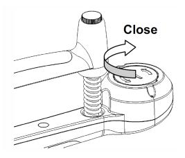
3)Lock the battery cover by turning clockwise.
