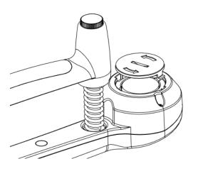
1) Remove the battery cover by turning anticlockwise.
