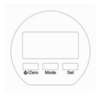
🖒 /ZERO : Power on / Power Off / Zero Press to Power On, hold for 3 seconds to Power Off.
