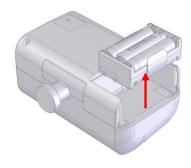
3. Remove the battery housing.
