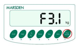
Press PRINT/ON/OFF, and F3.1 should appear on the screen. Press PRINT/ON/OFF again.
