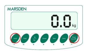
Press PRINT/ON/OFF once and HOLD twice to set the time out period and return to normal weighing mode.
